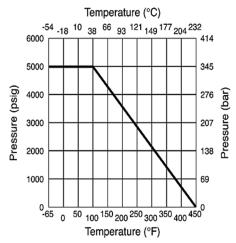
Legend: A - Stainless Steel with R stems; Note: To determine MPa, multiply bar by 0.1
